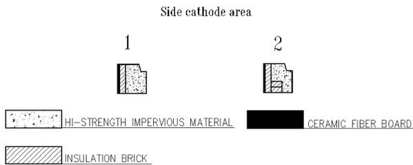
**Figure 6: Side wall area at block level**
