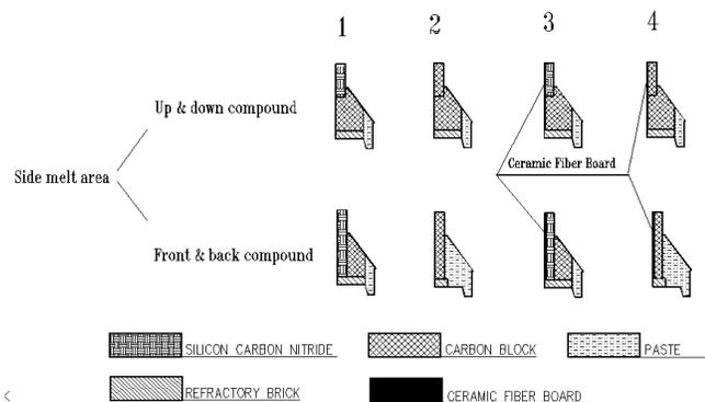
**Figure 3: Side wall area at liquids level**
