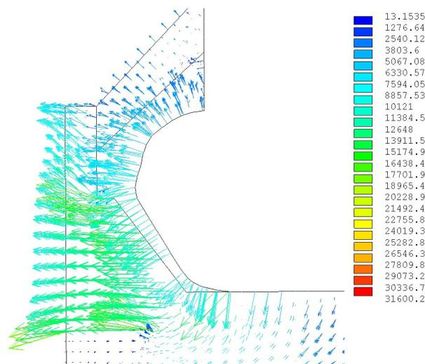
**Figure 5: Heat flux of side ramming paste**
